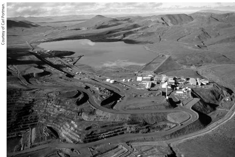
The Red Dog Mine. The open pit is in the lower left of the picture. Tailings lake and mill complex stretches across the picture. The road to the port leaves the picture in the upper left.
